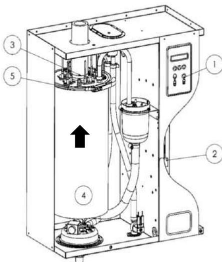
Fig. 6-1. Humidifier Stainless steel tank
