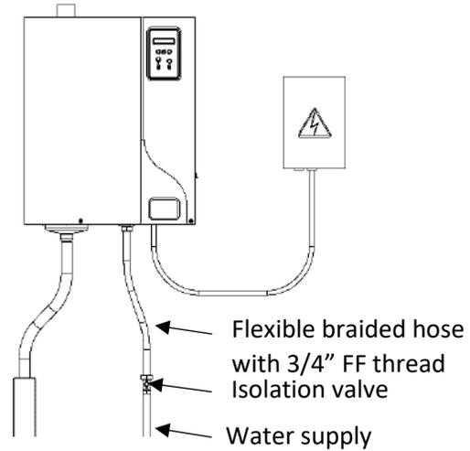
Fig. 3-2. Humidifier water supply
