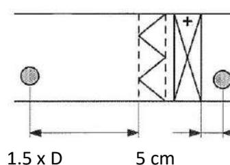
1.5 x D before a particle filter or absolute filter
