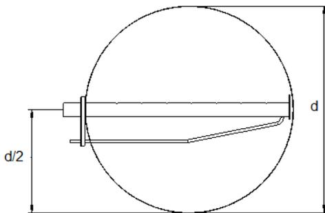
**Fig. H 3-3.  $d$  = Diameter of the duct**
