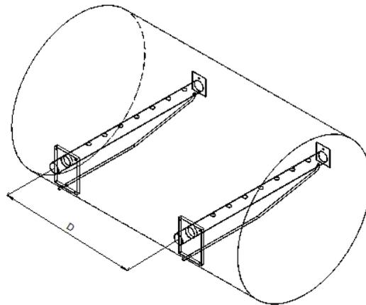
**Fig. I 3-3.  $D$  = Distance between two tubes**
