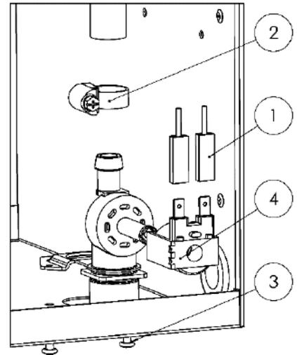
Fig. 6-3. Humidifier water inlet valve
