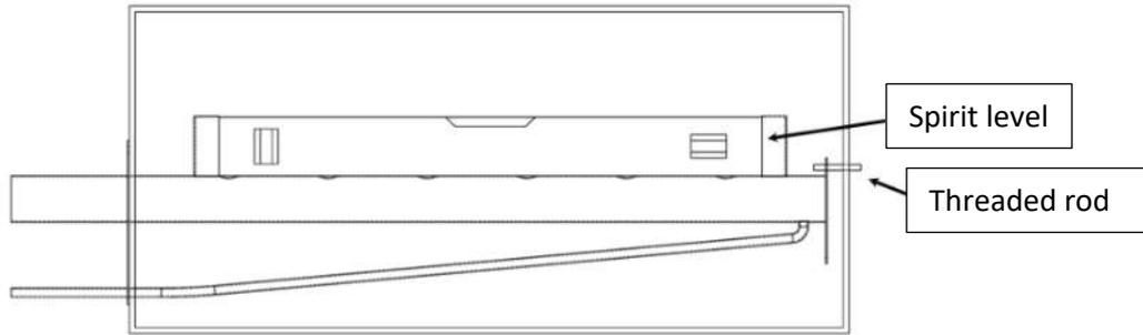
Fig. A 3-3. Steam dispersion tubes positioning
