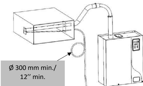
Fig. A 3-4. Standard installation
