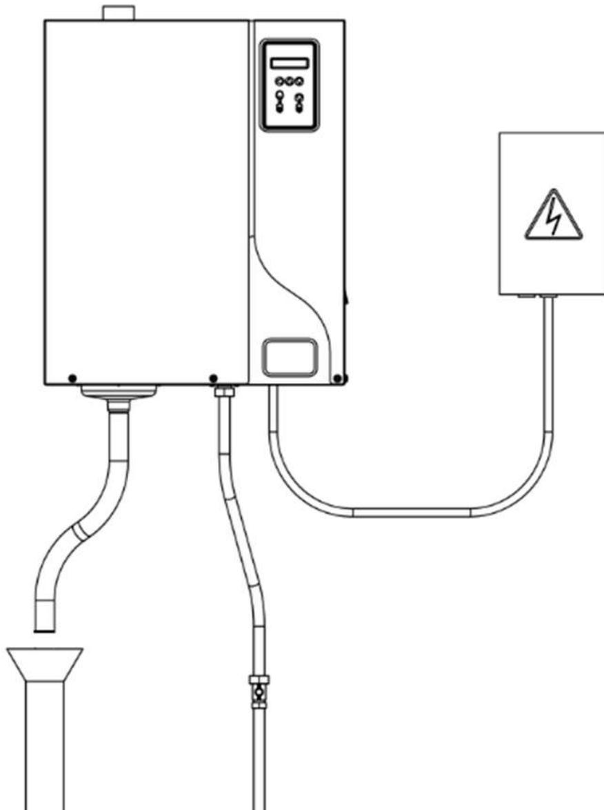
Fig. B 3-6. Example of Installation with funnel
