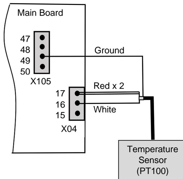
2. **Defective temperature sensor.** Disconnect the temperature sensor from connector X04. Use a multimeter to measure the resistance value of the PT100 at room temperature and compare this value with the PT100 resistance table.
