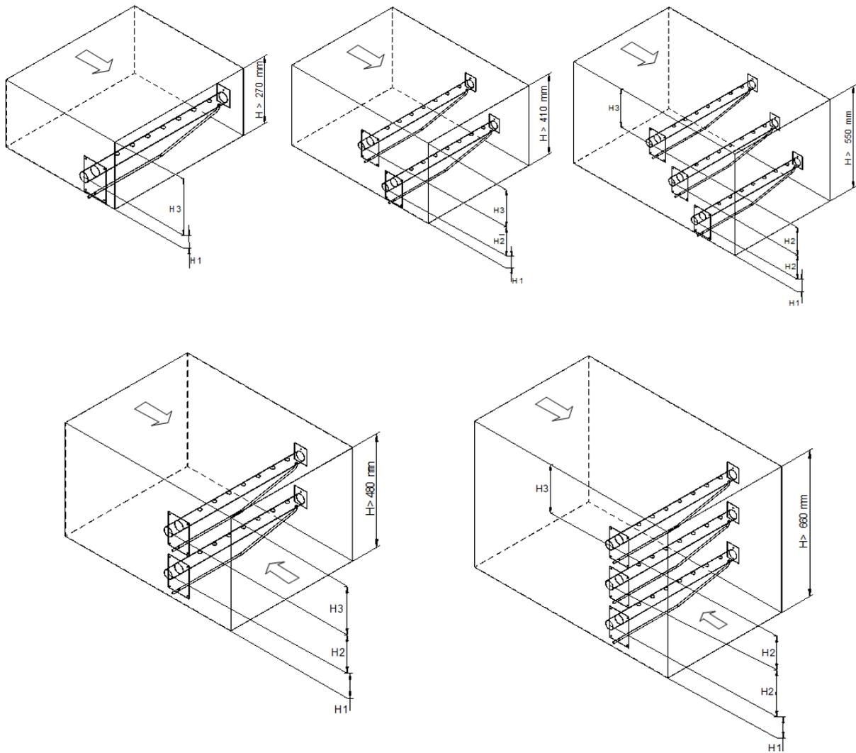
Fig. E 3-3. Minimum heights & flow directions
