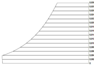
**1. Humidity ratio values** are plotted vertically along the right-hand margin, beginning with 0 kg/kg of dry air at the bottom and extending to 0,03 kg/kg of dry air at the top.
