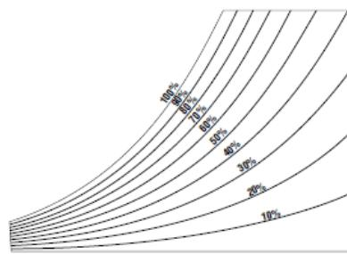
**5. Relative humidity** lines curve across the chart from left to right at intervals of 10%. They begin at the bottom at 10% and end at the top with the saturation curve (100%).
