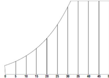
**3. Dry-bulb temperature lines** are plotted vertically at 1°C intervals.
