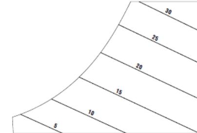
**4. Wet-bulb temperature lines** are indicated obliquely and fall almost parallel to enthalpy lines. They are shown at 1°C intervals.
