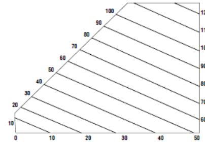
**2. Enthalpy**, or total heat, is plotted with oblique lines, at intervals of 10 kJ/kg of dry air, extending from upper left to lower right.
