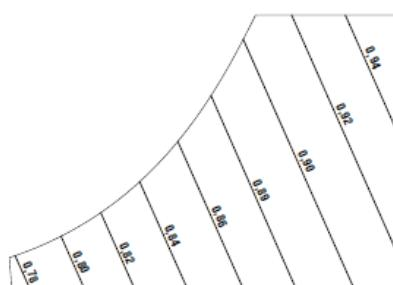
**6. Volume** lines indicating cubic meter per kilogram of dry air are plotted at intervals of 0,01 m³.
